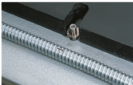
Cut longitudinally across 2 hose covering segments
