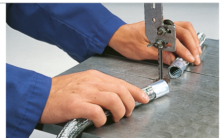
Conduit ends are clean without splaying, due to adhesive tape binding
