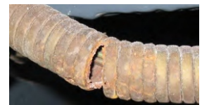
Metal Core Corrodes Limited Service Life
