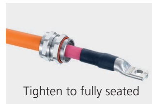
4. Tighten the pressure nut
