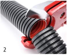
Use a suitable tool (cutter or ROHRflex scissors) to cut the ROHRflex corrugated conduit straight through the
