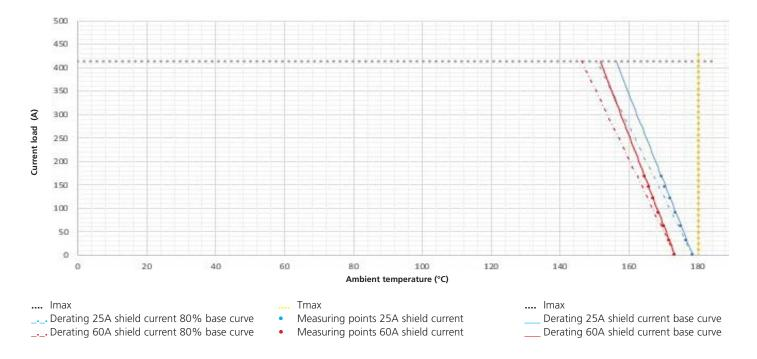
The **derating** diagram shows the permissible DC conductor load of a specific conductor depending on the ambient temperature for the defined DC shield currents. The conductor and shield load must be adjusted depending on the ambient temperature in order to avoid excessive temperature increases.
