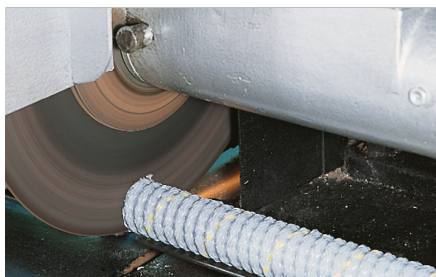
Position conduit below cutting disc (90°)
