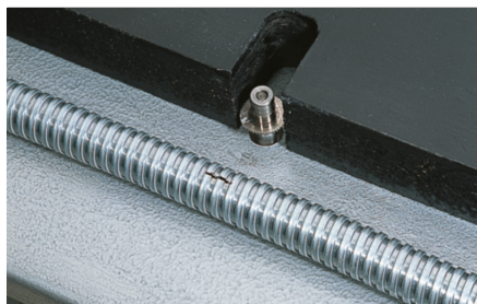
Cut longitudinally across 2 hose covering segments
