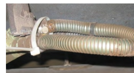
PVC Jacket Degrades Limited Service Life
