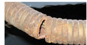
Metal Core Corrodes Limited Service Life
